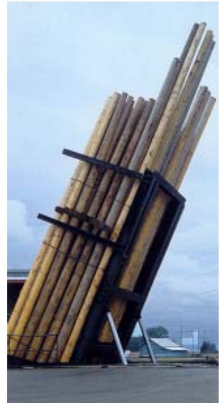
Butt-treatment in a tilt-up dip tank.
