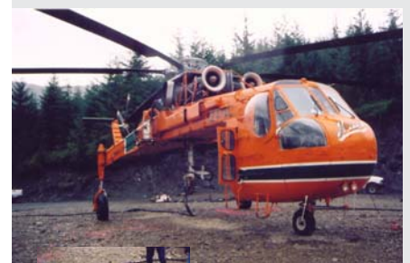
This helicopter with the grapple has a capacity to lift 18,000 lbs.
