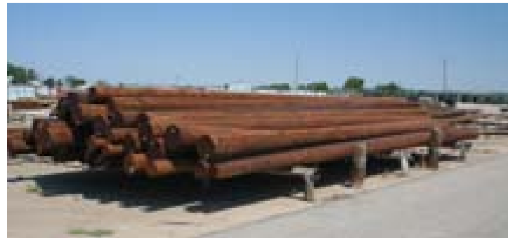
Morgan County REA maintain a good inventory of cedar poles in their yard. They use full-length, pentachlorophenol treated poles.
